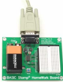
Figure 1-30 BASIC Stamp HomeWork Board Ready to Program
