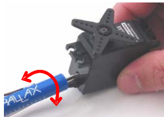
Gently turn screwdriver to adjust potentiometer
